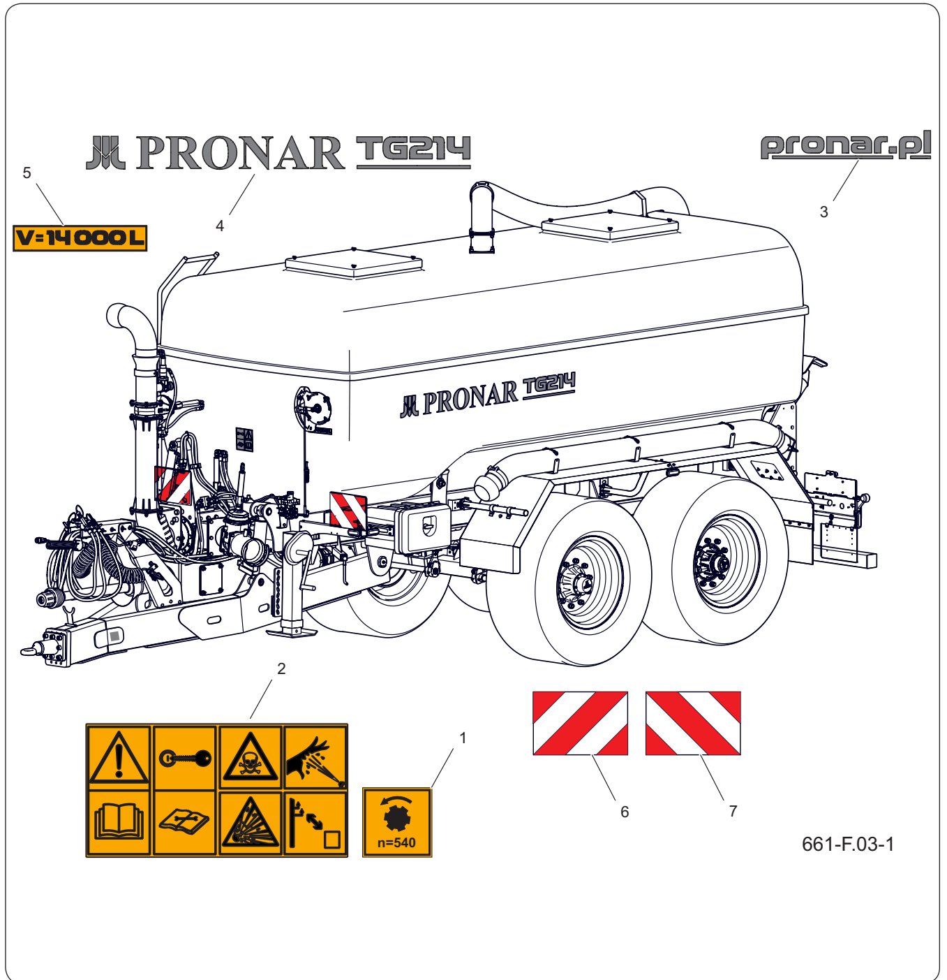
Figure 3.3 Positioning of information and warning stickers
