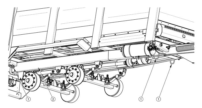
FIG. 1.3 Positioning of transport lugs
