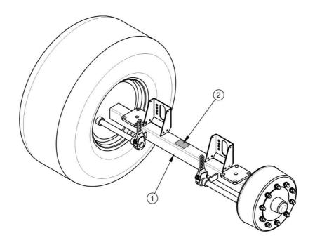
FIG. 1.2 Location of the axle data plate
