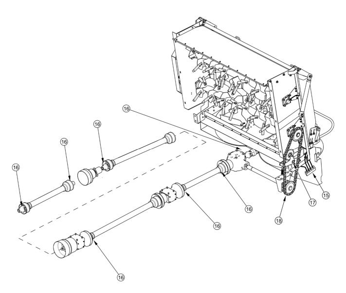
FIG. 5.13 Spreader's lubrication points N262, N262/1
