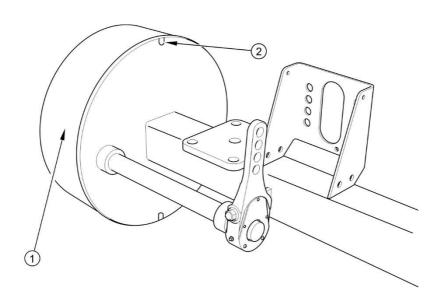
FIG. 5.1 Checking brake shoe linings
