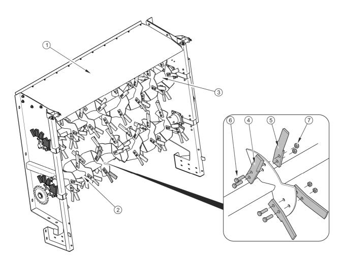
FIG. 5.15 Replacement of the disintegrating knives of the spreader unit mechanism
