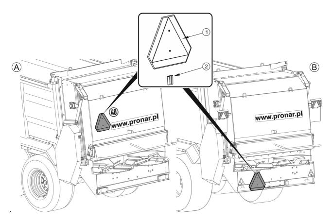
FIG. 2.2 Positioning the warning sign
