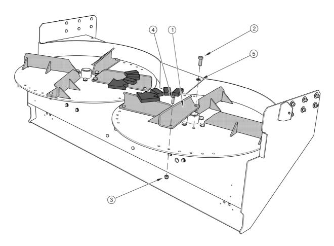
FIG. 5.14 Replacing spreading disc blades
