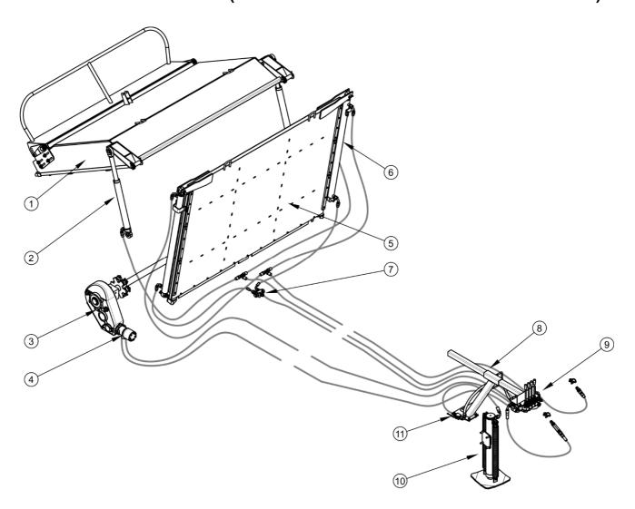
FIG. 3.7 Hydraulic system design (system controlled from the manure spreader)
