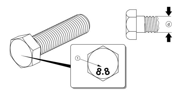
FIG. 5.19 Bolt with metric thread
