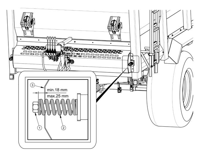
FIG. 5.16 Adjusting the floor chain tension
