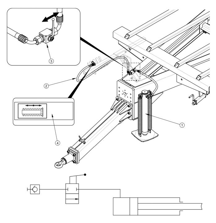
FIG. 3.4 Straight support hydraulic system construction and diagram
