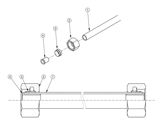
FIG. 5.10 Installation of the pneumatic line
