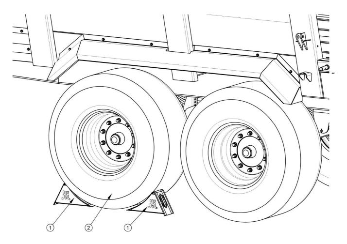
FIG. 2.1 Method of placing chocks
