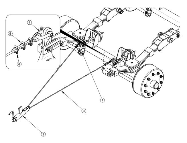
FIG. 5.6 Adjustment of parking brake cable tension
