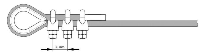
FIG. 5.7 Installation of steel cable clamps
