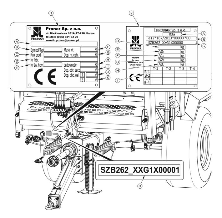
FIG. 1.1 Manure spreader identification
