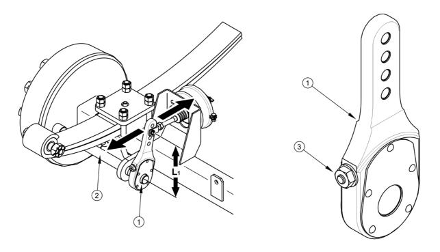
FIG. 5.5 Adjustment of axle mechanical brakes
