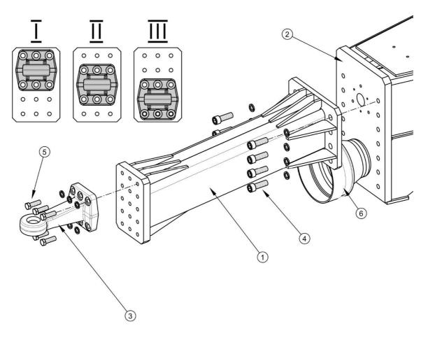
FIG. 5.17 Mounting the upper drawbar
