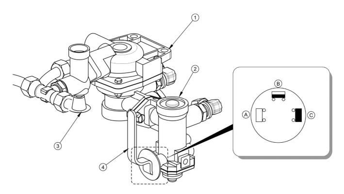
FIG. 3.15 Control valve and brake force regulator
