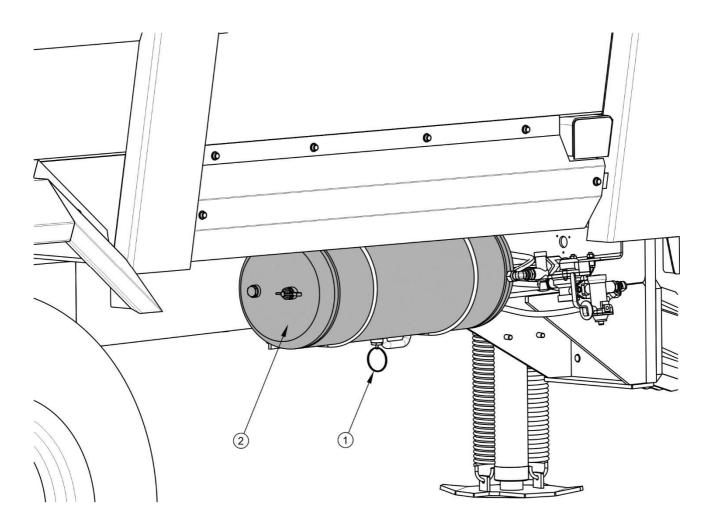
FIG. 5.9 Draining water from air tank
