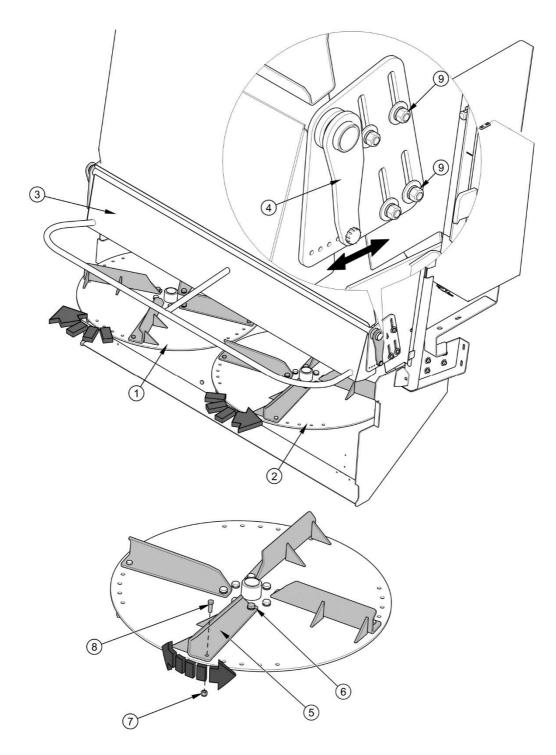
FIG. 4.4 Adjustment of spreading width
