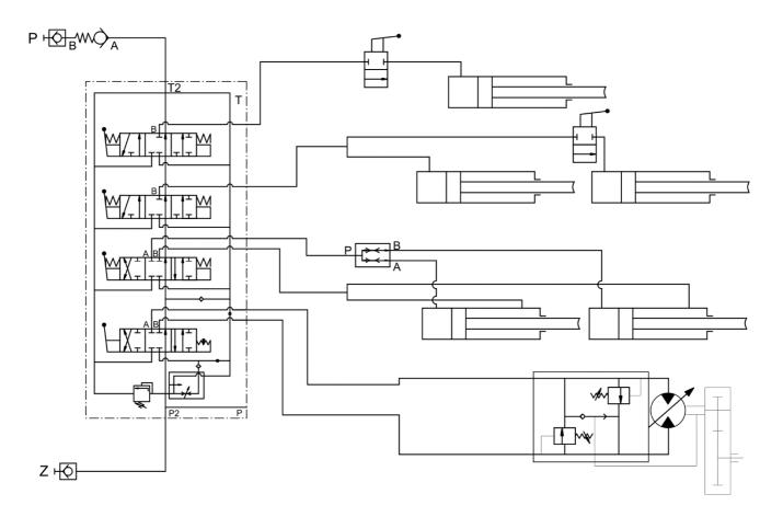
FIG. 3.9 Hydraulic system diagram (system controlled from the manure spreader)
