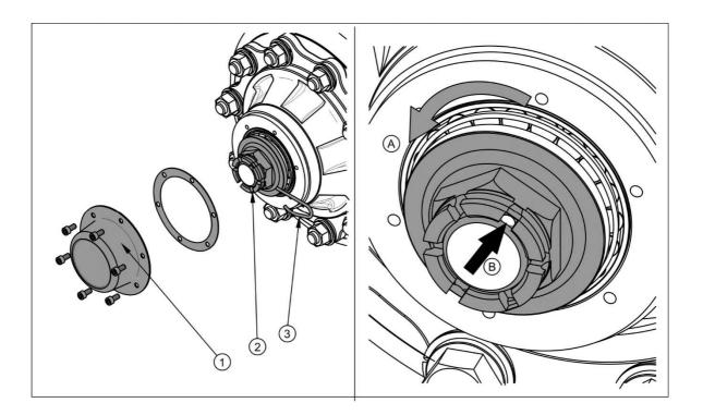
FIG. 5.3 Adjustment of road wheel axle bearings
