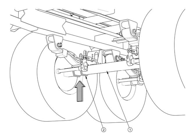
FIG. 5.2 Lifting jack support point
