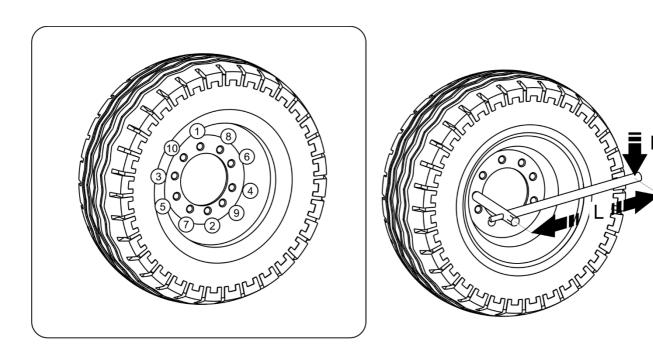
FIG. 5.4 Sequence of tightening nuts, axles with 10 M22x1.5 pins
