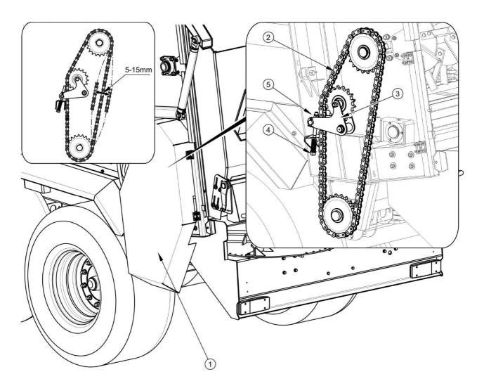
FIG. 5.18 Adjusting the chain transmission
