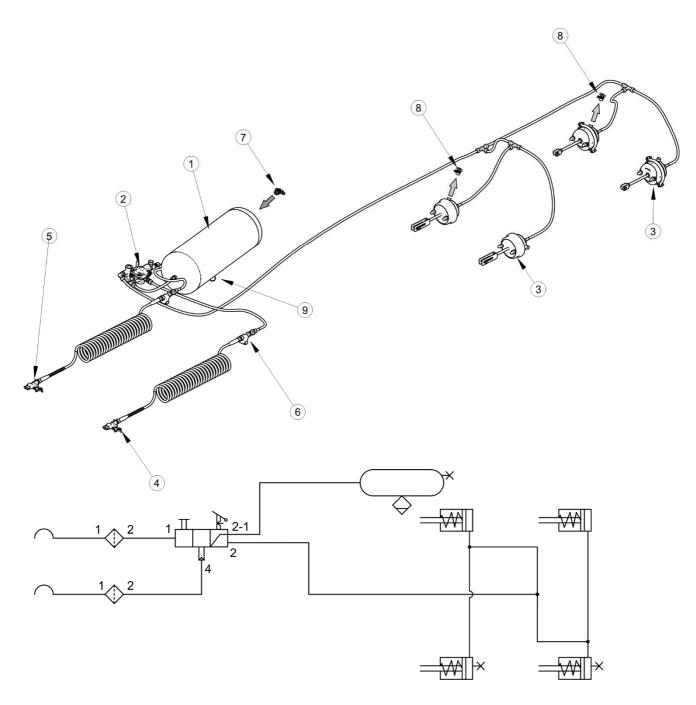
FIG. 3.12 Double line pneumatic system
