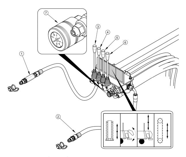
FIG. 3.8 Hydraulic selective control valve
