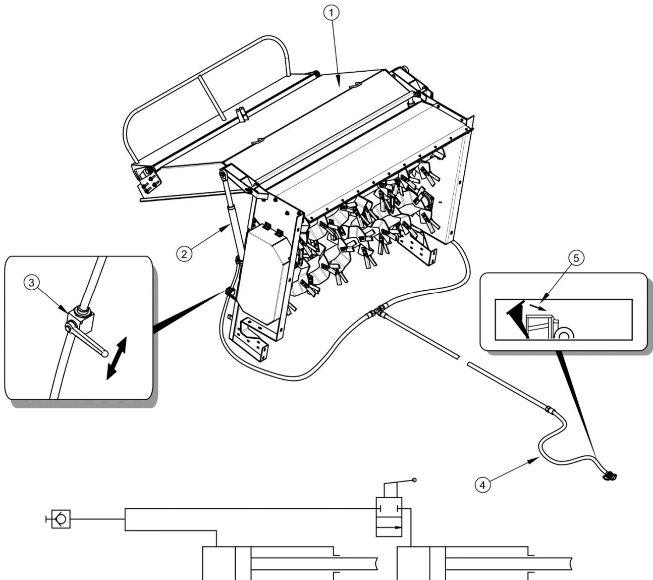
**FIG. 3.5 Tailgate hydraulic system construction and diagram**
