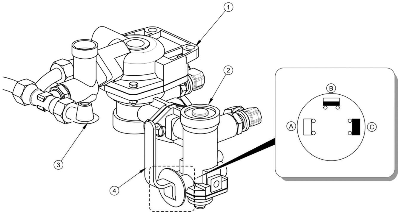
**FIG. 3.15 Control valve and brake force regulator**
