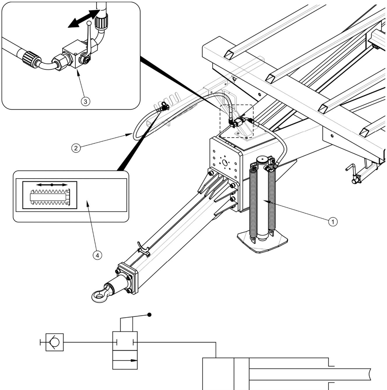
**FIG. 3.4** Straight support hydraulic system construction and diagram
