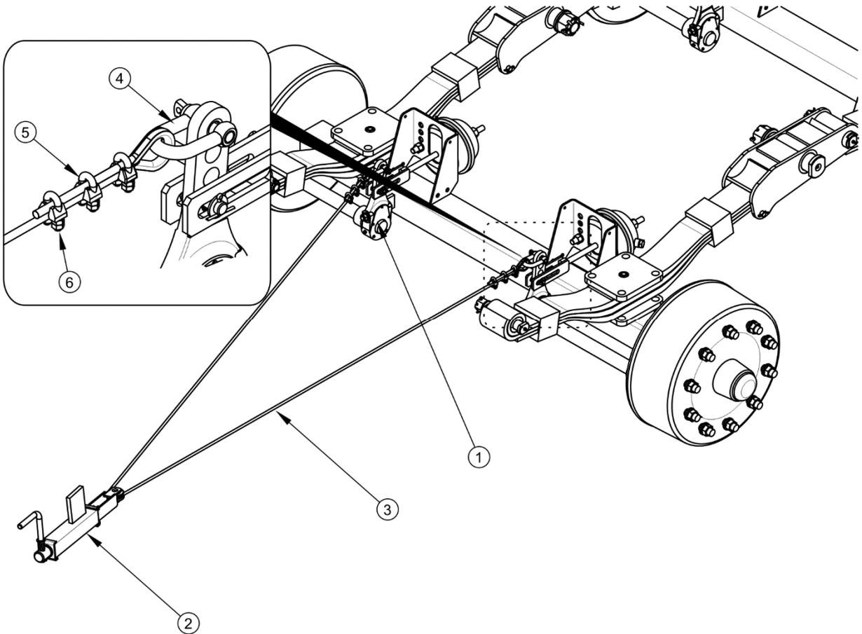
**FIG. 5.6 Adjustment of parking brake cable tension**
