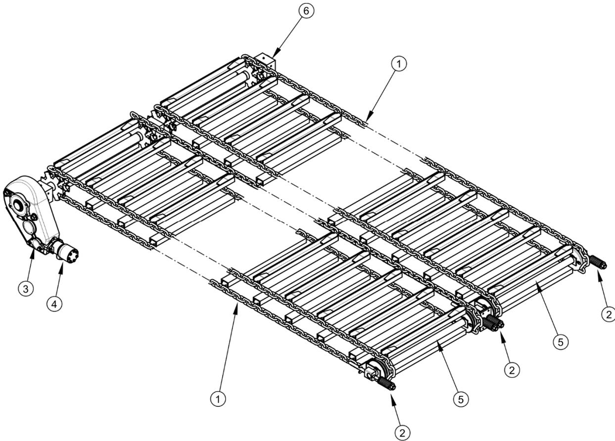
**FIG. 3.2 Feeding mechanism**
