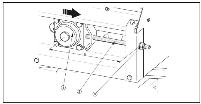
FIG. 5.8A Adjustment of conveyor belt tension
