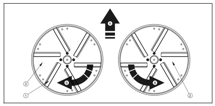
FIG. 3.5A Spreading adapter discs
