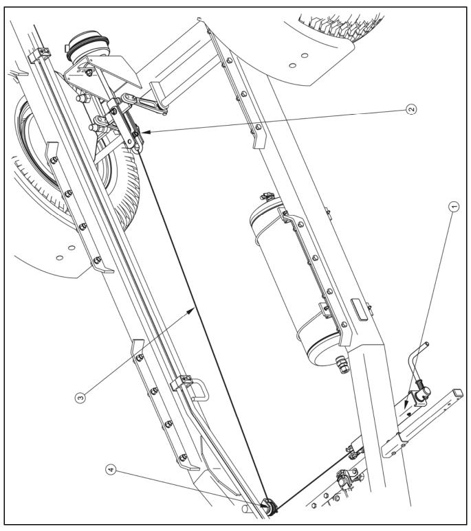
FIG. 3.12A Parking brake of sand spreader
