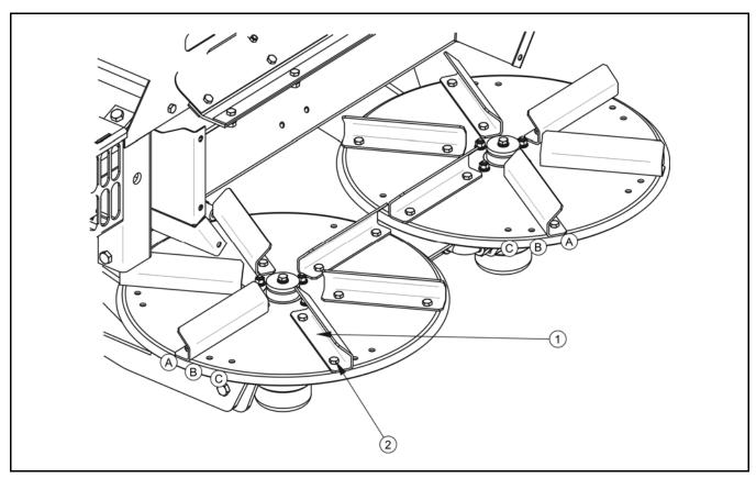
FIG. 5.9A Changing rake angle of blades
