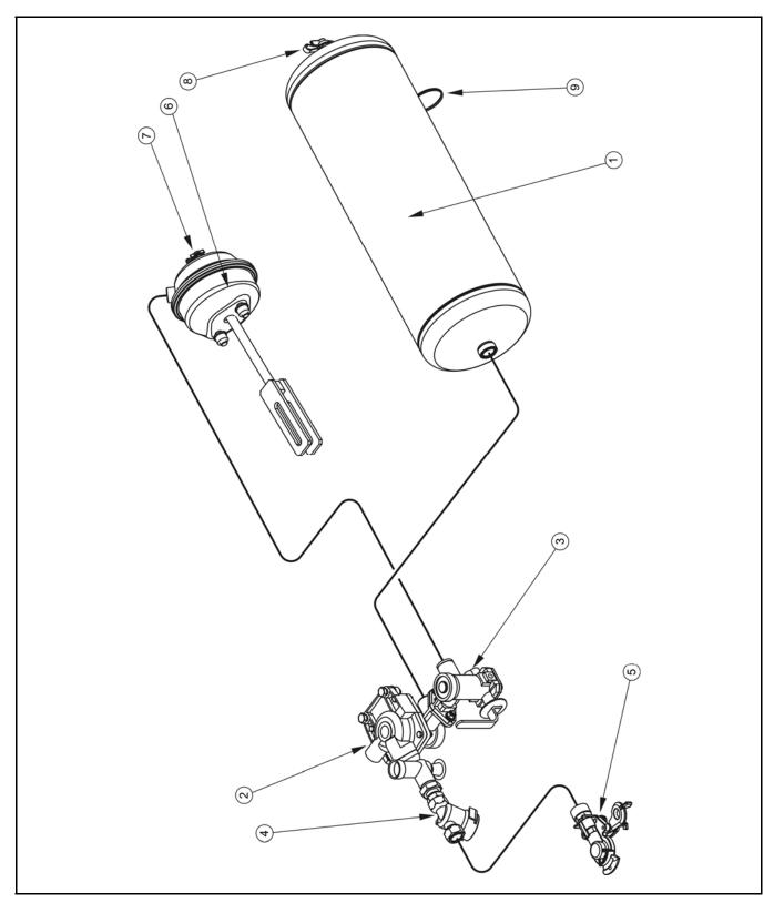
FIG. 3.9A Single conduit pneumatic system
