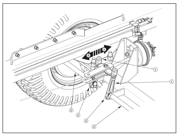
FIG. 5.3A Adjustment of main brakes
