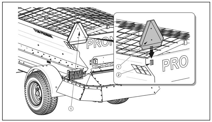
FIG. 4.7A Attaching a slow-moving vehicle warning sign
