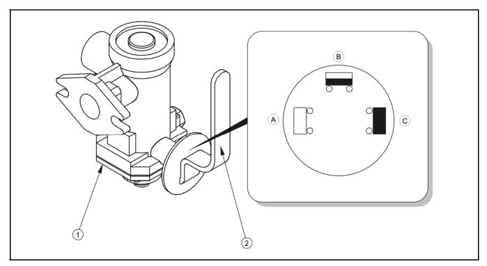
FIG. 3.11A Three-step brake force regulator
