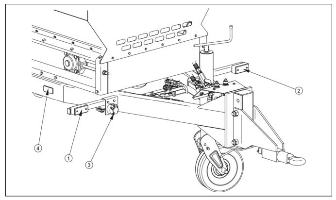
FIG. 3.13A Positioning of electrical components and reflective lights, front view
