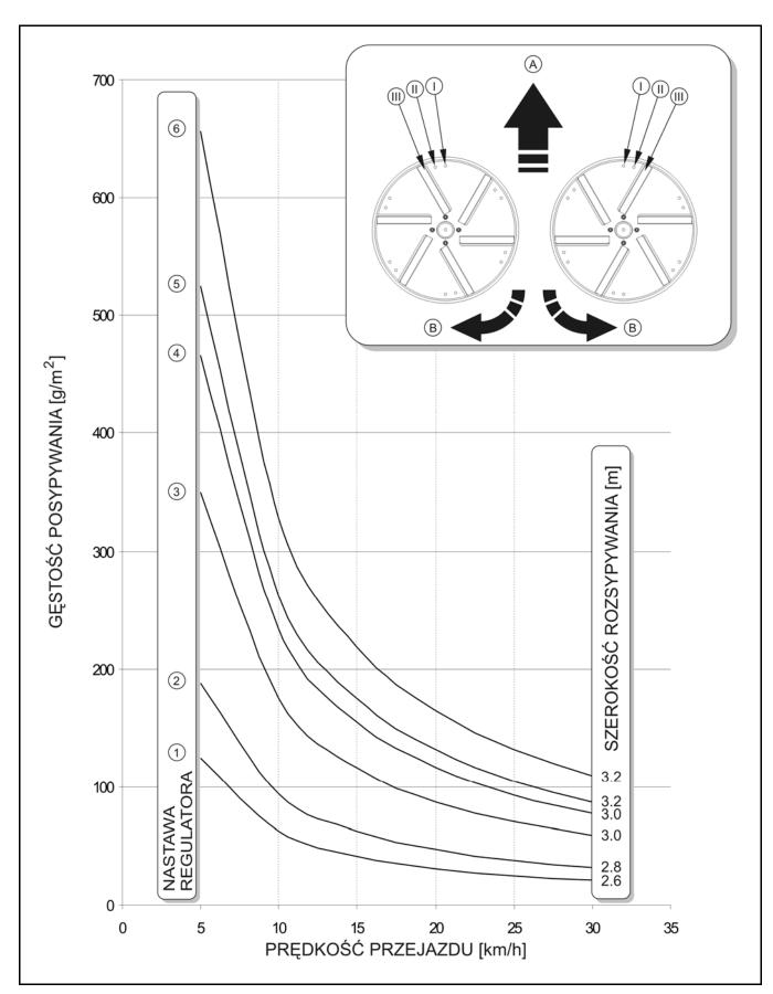
FIG. 4.6A Spreading density, diagram 3
