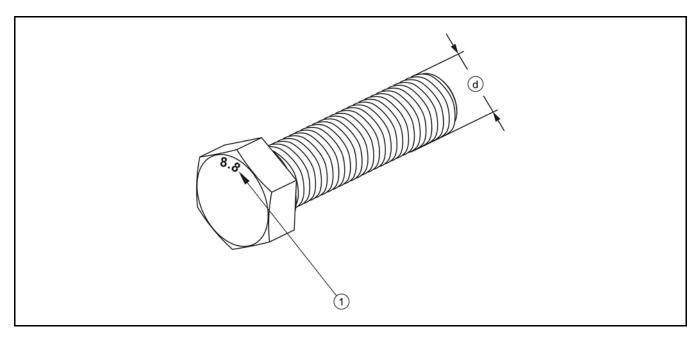
FIG. 5.11A Bolt with metric thread
