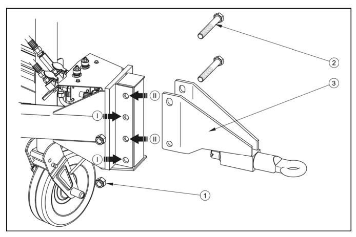
FIG. 5.1A Adjustment of drawbar position
