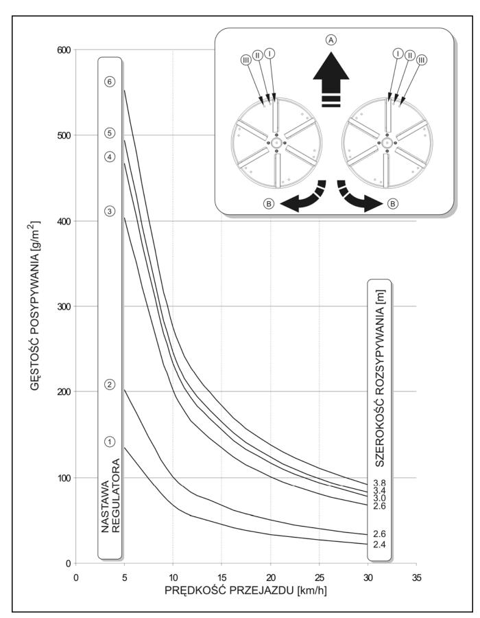
FIG. 4.4A Spreading density, diagram 1
