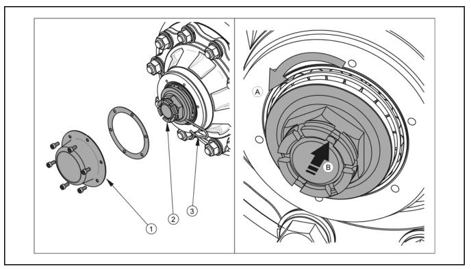
FIG. 5.2A Adjustment of road wheel axle bearings
