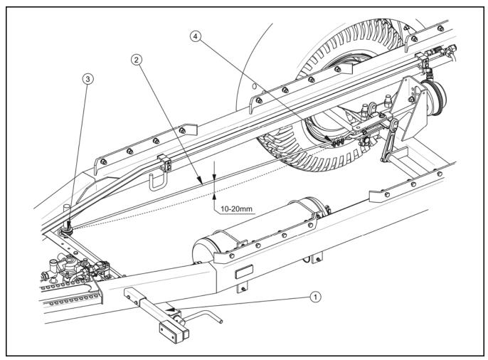
FIG. 5.4A Parking brake adjustment
