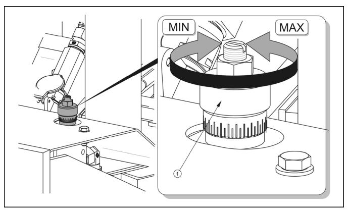
FIG. 4.3A Adjustment of conveyor belt speed
