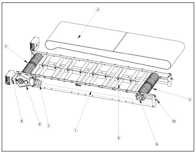
FIG. 3.3A Feeding mechanism
