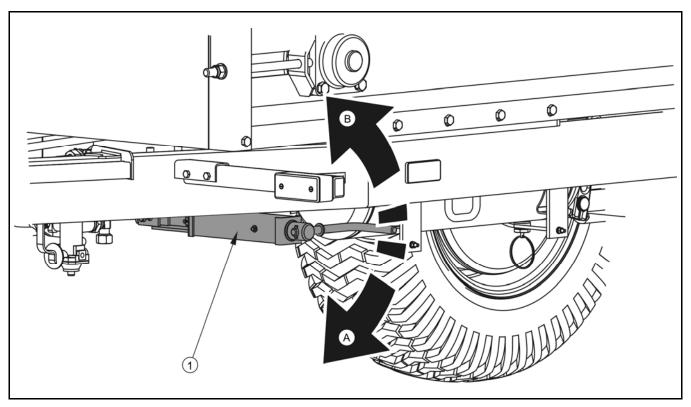
FIG. 4.2A Parking brake mechanism
