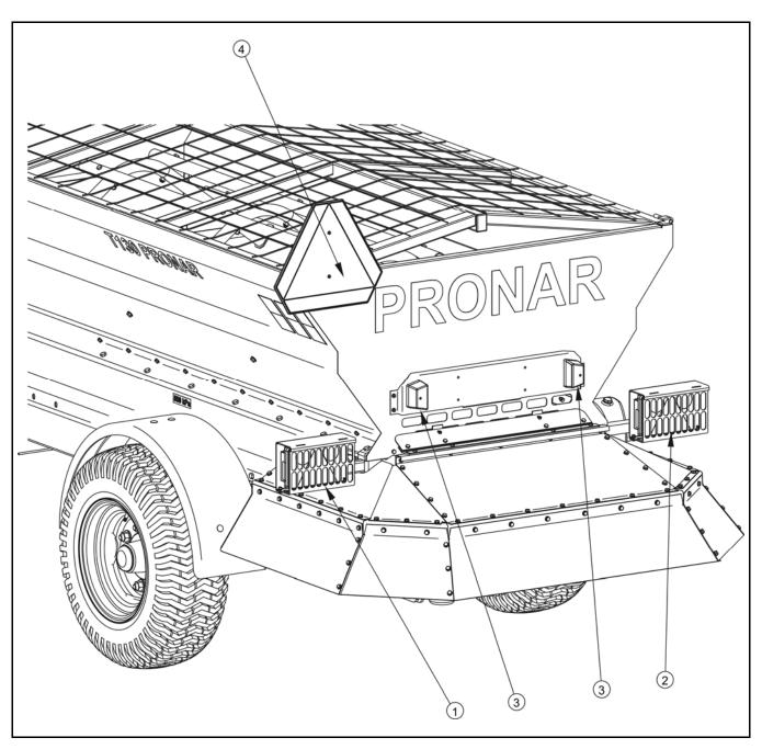
FIG. 3.14A Positioning of electrical components and reflective lights, rear view
