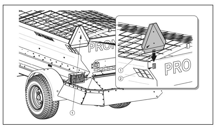
FIG. 2.1A Positioning the warning sign
