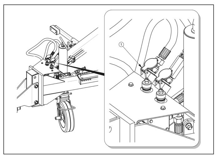
FIG. 4.8A Sockets for hydraulic conduit plugs
