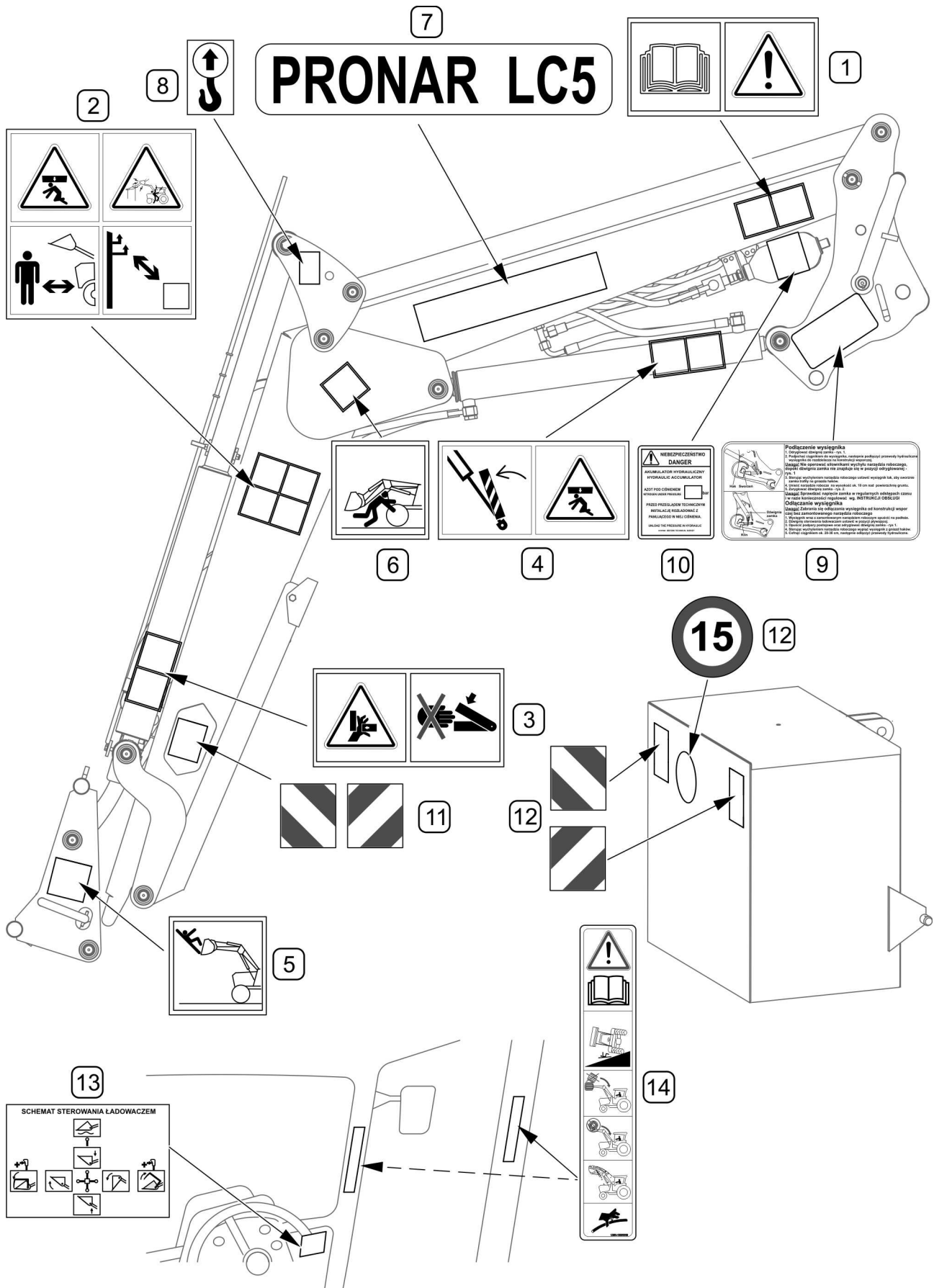
FIGURE 2.1. Arrangement of information and warning stickers
