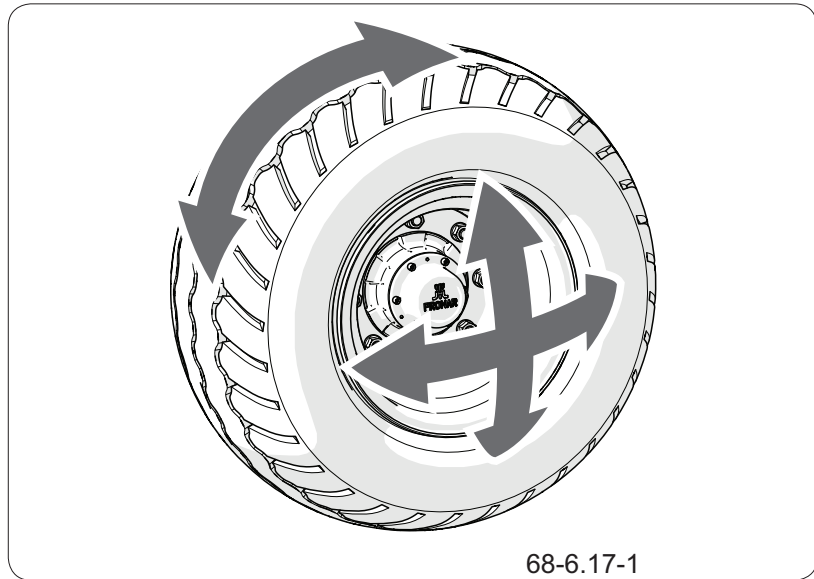
Figure 6.6 Check wheel half axle bearings looseness
