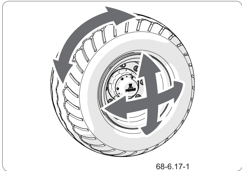
Figure 6.6 Check wheel half axle bearings looseness
