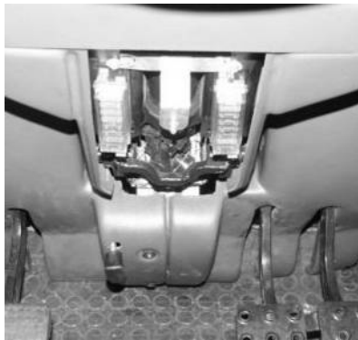
Fig. E-28 Location of fuses FB1 and FB2 near steering column. A- bolts; B- cover
