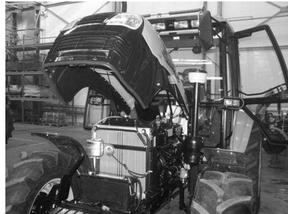
Fig. E-30 Engine bonnet. 1 – engine bonnet; 2 – pull rod of the bonnet lock
