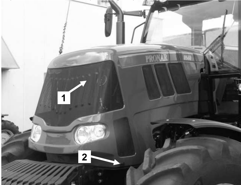
Figure 5-38 Bonnet and engine side covers. 1 - engine bonnet; 2 - bonnet catch release
