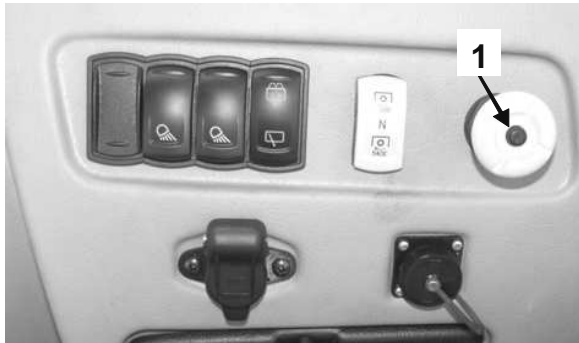
Figure 4-30 PTO activation switch on PRONAR tractors and method of engaging PTO drive. 1- rear PTO switch
