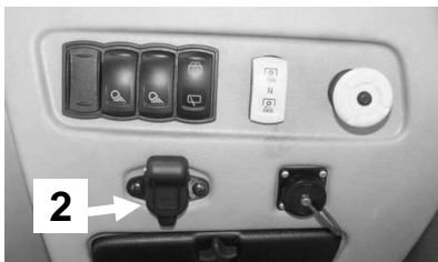
Figure 5-30 Connection 1 of electrical system and socket 2 for supply +12V 20A to additional receivers connected to tractor electrical systems.
