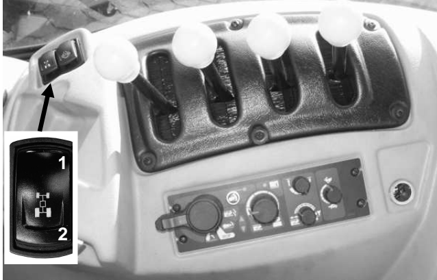
Figure 4-26 Front axle drive connector may be set in two positions:
