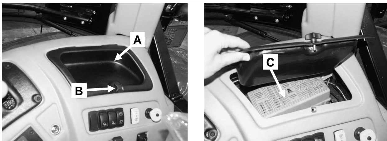
Figure 5-34 location of certain fuses and switches on the right above the wheel. A- screw; B- cover; C- fuse and relay box.
