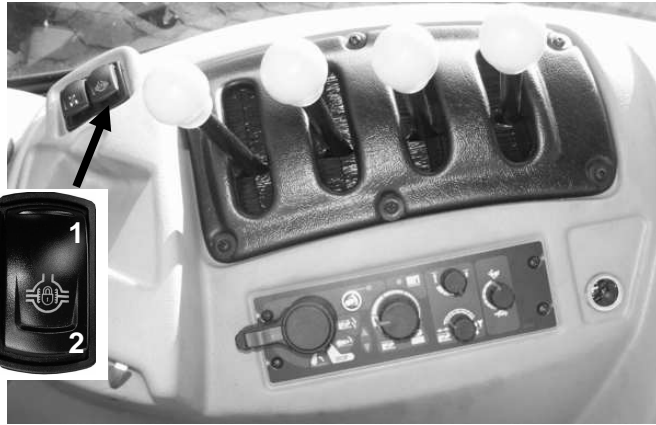
Figure 4-27 Front axle differential lock mechanism control (located on switch panel on the right side of the seat)
