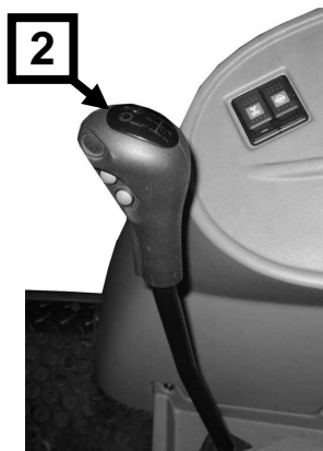
Figure 5-6. Travel direction switch and gear lever of PRONAR 6170 / 6180 tractors.
