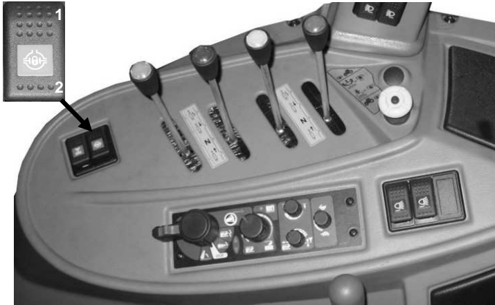
Figure 4-27 Front axle differential lock mechanism control (located on switch panel on the right side of the seat)
