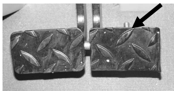
Figure 4-24 Catch locking working brake pedals.
