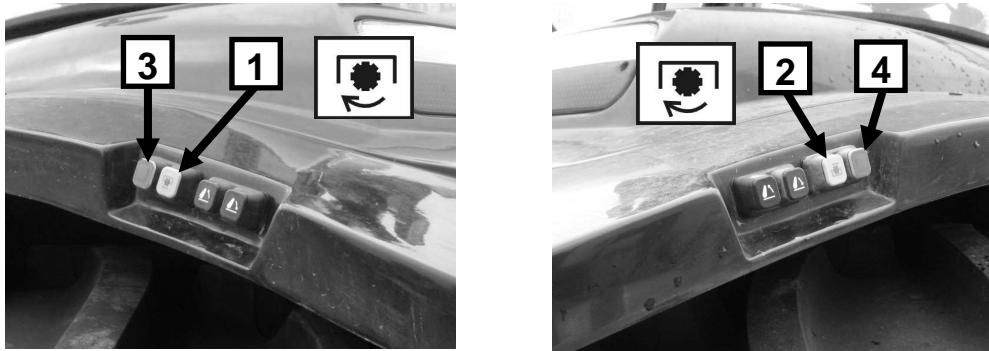
Figure 4-31 PTO switch on left 1 and right 2 rear tractor mudguard and PTO switch on left 3 and right 4 rear tractor mudguard.
