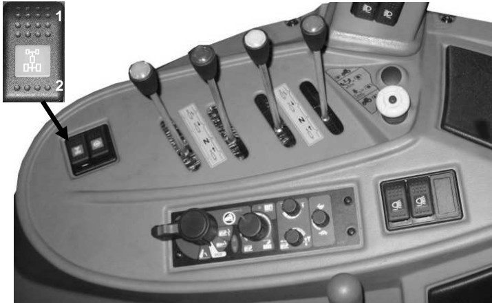
Figure 4-26 Front axle drive connector may be set in two positions: 1 - drive disengaged (upper); 2 - drive engaged (lower).
