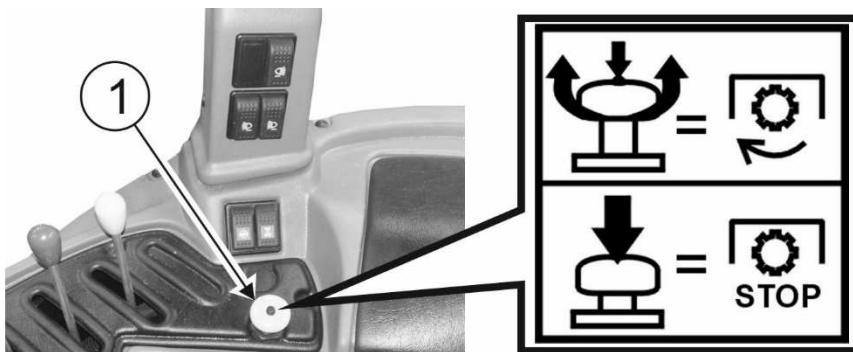
FIGURE 3.35 PTO switch inside the tractor cab (on the console on the right side of the seat).
