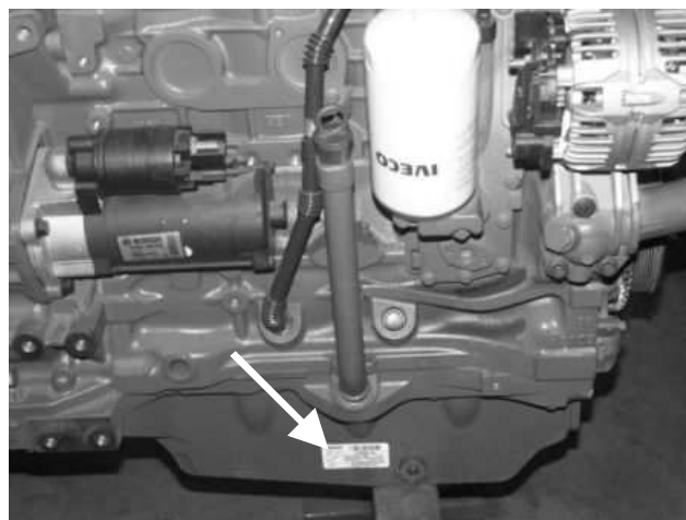
Figure 3-2a Location of IVECO engine rating plate (on oil tank, on the right side of engine)
