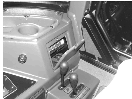
Figure 5-35 location of fuse set FB3 on the right above the wheel. A - screw; B - cover
