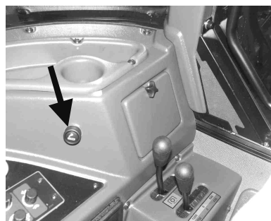
Figure 5-30 Connection of electrical system for trailers 1 and +12V supply socket to supply additional receivers connected to tractor electrical systems 2 .
