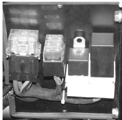
Figure 5-35 location of fuse set FB3 on the right above the wheel. A - screw; B - cover
