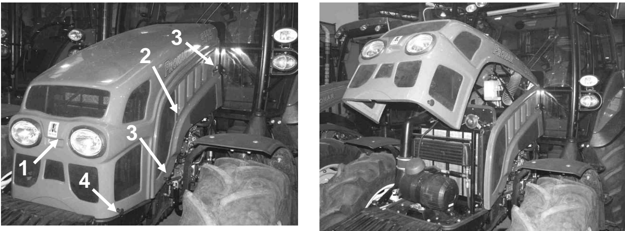
Figure 5-41 Bonnet and engine side covers. 1 - engine bonnet; 2 - side cover; 3 - snap fasteners securing side cover; 4 - bonnet lock release pull rod
