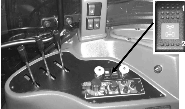
Figure 4-27 Front axle drive connector may be set in two positions:
