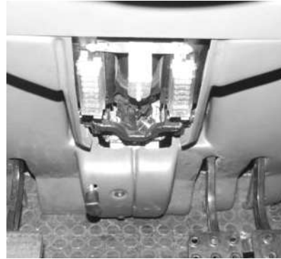
Figure 5-34 Position of fuse sets FB1 and FB2 by steering column. A - screw; B - cover
