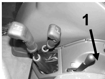
Figure 5-6 Reducer lever- setting. 1 - slow "field" gears; N - neutral; 2 - fast "road" gears.
