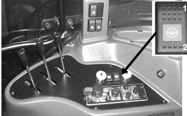
Figure 4-28 Rear axle differential lock mechanism control (located on switch panel on the right side of the seat)
