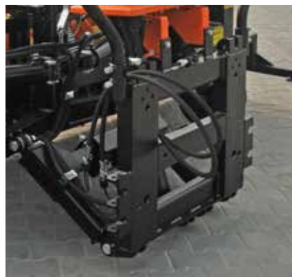
Montage – plaque municipale DIN de type A
