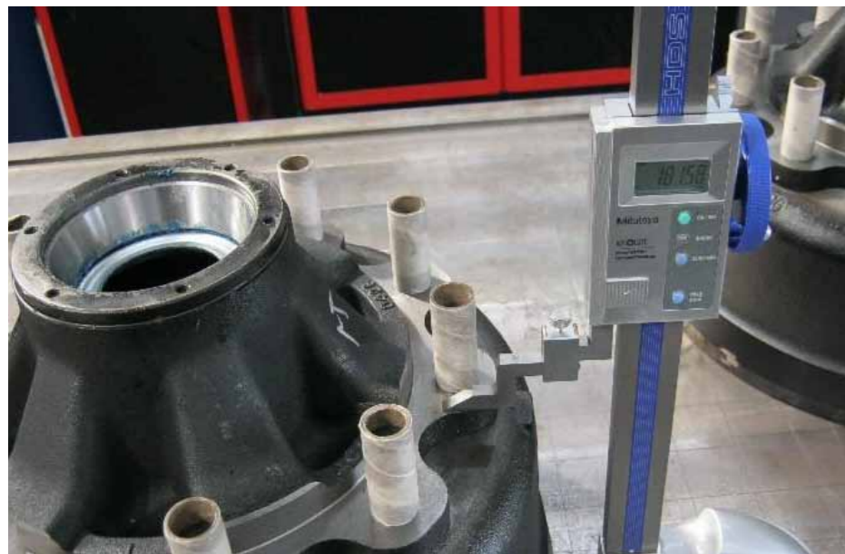
Example of hub drum dimension measurements. On the left: the distance from the drum end to the hub using a height gauge (181±1 mm); on the right: measurement of the location of the bearing race using a depth gauge (114±1 mm)
