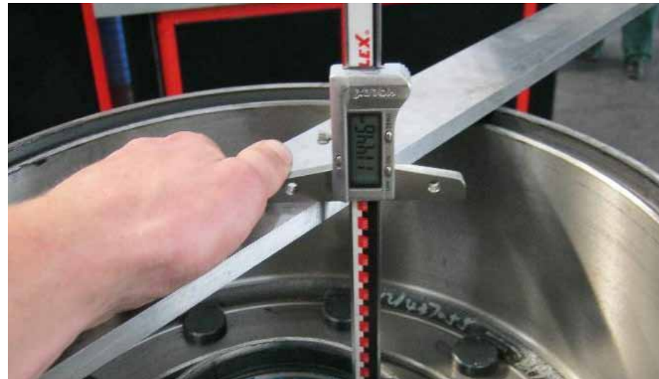
Example of hub drum dimension measurements. On the left: the distance from the drum end to the hub using a height gauge (181±1 mm); on the right: measurement of the location of the bearing race using a depth gauge (114±1 mm)
