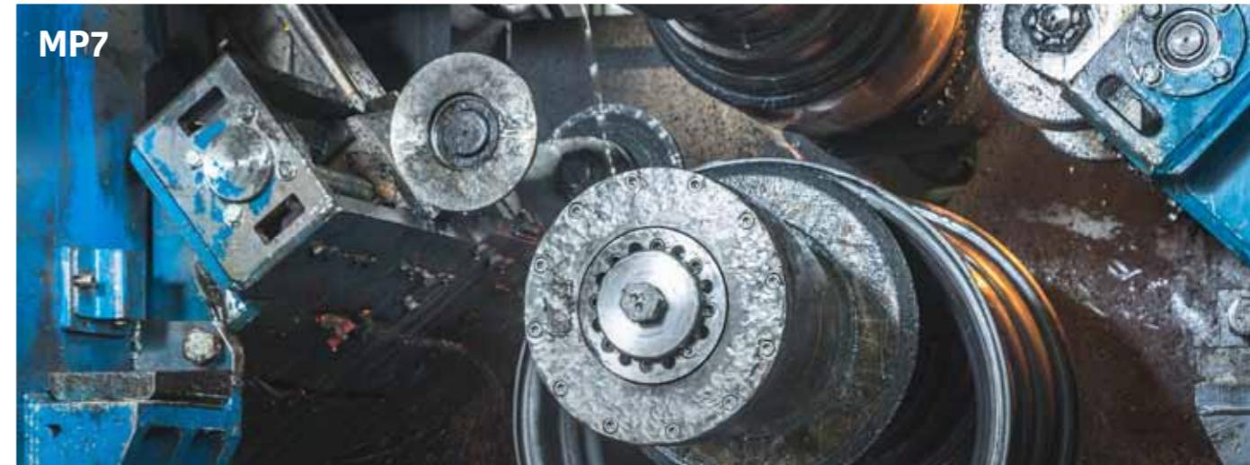
Designed and produced at PRONAR the production line for profiling bare rims enables us to meet the needs of even the most demanding customers by the ability to manufacture bare rims up to 10mm thick, in automatic cycles while maintaining the highest quality standards. The key to this success is a high degree of accuracy and repeatability of machine positioning.
