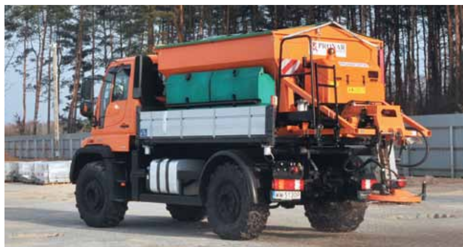
Posypywarka SPT40 na platformie MB Unimog
